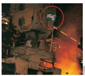
Multipin Plugs & Sockets are used in harsh environment like steel mills.
