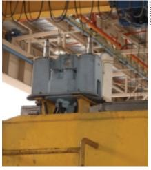
PSA in Singapore use the "Rackmatic" system for their Pasir Panjang terminal (PSA) where they needed a fully automatic connector for fast changes of the spreaders.
