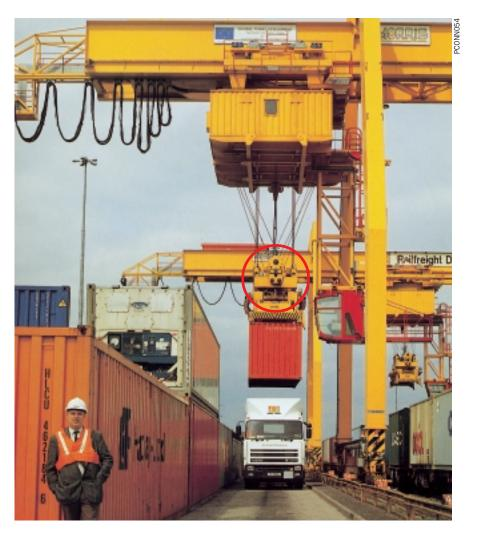
A typical application for spreader connector type "Rackmatic"
