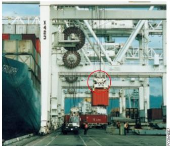
Plugs & Sockets of Push & Pull type are used to connect quickly and easily on various crane equipment like spreaders, vacuum-loaders, hydraulic grabs and other crane lifting equipment. The photo shows a typical application area.
